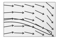
Figure 3: Optimal SMA fiber path and direction of the principal stress.
