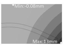
Figure 4: Displacement distribution when SMA fibers are activated.
